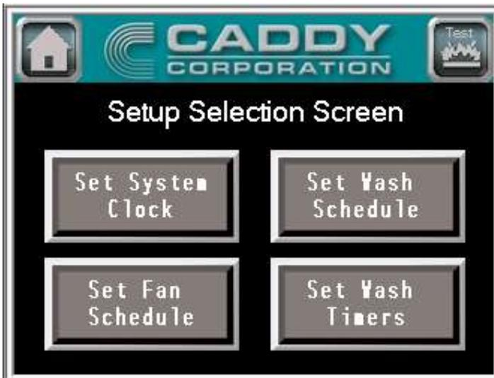
To get to the Setup Selection Screen press the **Login** button and login. Pressing either of the four buttons will take you to the screens shown below.
