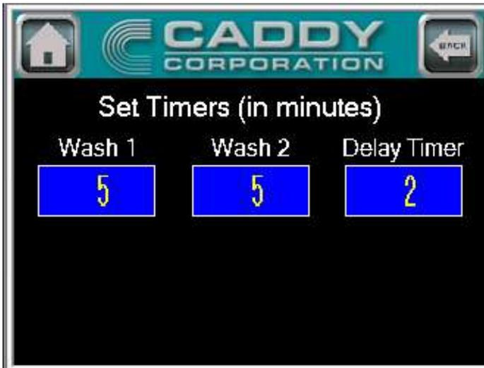
The amount of wash timers that show up on this screen is directly related to the amount of wash sequences that are wired to the PLC. If only 1 is wired, then 1 timer shows up. If 4 are wired, then 4 timers show up. By pressing the number shown below the Wash Title you can set the duration in minutes of the wash cycle.
