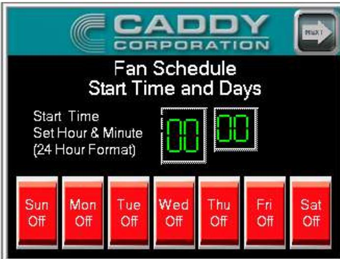
Using the schedule is not a necessity, but if desired, you can set the fan start time and days on this screen. Use military time to set the desired start time and press each day you wish to run the fans. The days will turn green and say "Sun On" and so on, for each selected day. You will set the stop time in the next screen.
