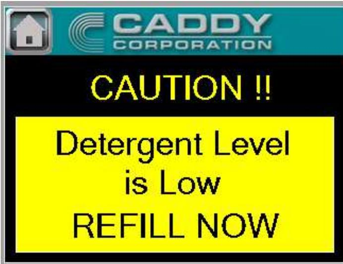
The water wash control panel is provided with a detergent reservoir. There is a float switch inside of the reservoir that will send a signal when the detergent needs to be replaced. The screen will show the Refill Now screen. When the **Home** button is pushed it will change to back to the Home Screen and a Low Detergent indicator will flash in the **Fan Stop Start Wash** button.
