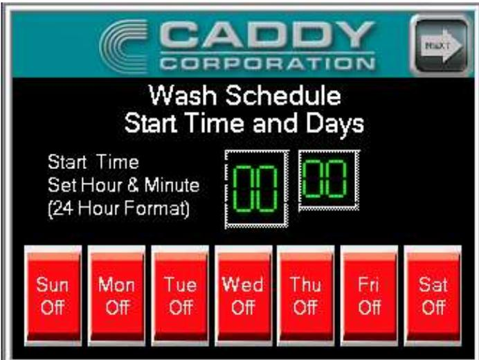
Since the wash cycle runs at the end of the day you are essentially scheduling the fan stop time and the wash time at the same time. Using the criteria listed above, program the desired fan stop time and days.
