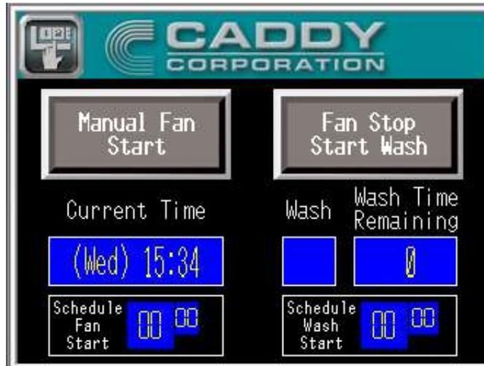
**Manual Fan Start:** When cooking operations occur the exhaust fans can be started by pressing the **Manual Fan Start** button. When activated the button will turn green and say **Fans Running**.
